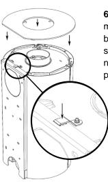
6. Secure the stove by mounting the safety bracket on top of the stove again. You can now remount the top plate.
