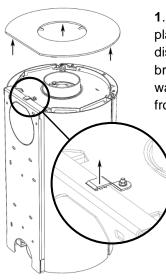
1. Dismount the top plate. Afterwards, dismount the safety bracket and pull the wall bracket away from the stove. **2**. Dismount the heat shield.
